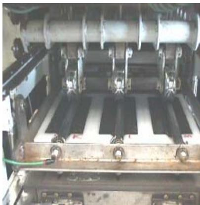
**Asphalt specimens being tested in the Asphalt Pavement Analyzer**
