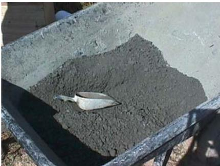
**Before placement, The RCC appears damp and has no liquid paste.**
