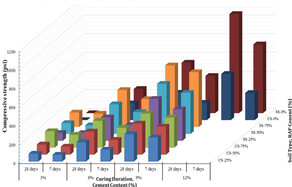
**Figure 2: Influence of Curing Duration on Compressive Strength of CMRB and S-C at Various Cement Contents**
