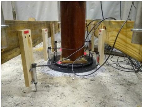
**Figure 1: Photo of Test Pit Load Plate Assembly**
