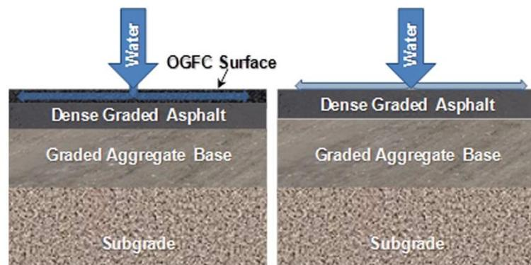
Illustration of water flow for a pavement with an OGFC layer (left) and without OGFC (right)
