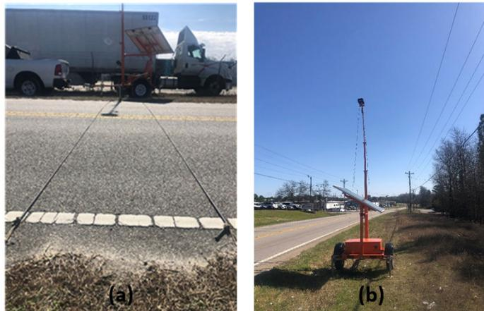
Figure 1. Methods to collect traffic data: (a) intrusive - using pneumatic tubes, (b) non-intrusive – using thermal camera and trailer
