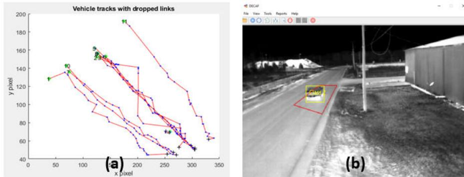
Figure 2. DECAF functionalities: (a) vehicle tracks, (b) vehicle detection and classification
