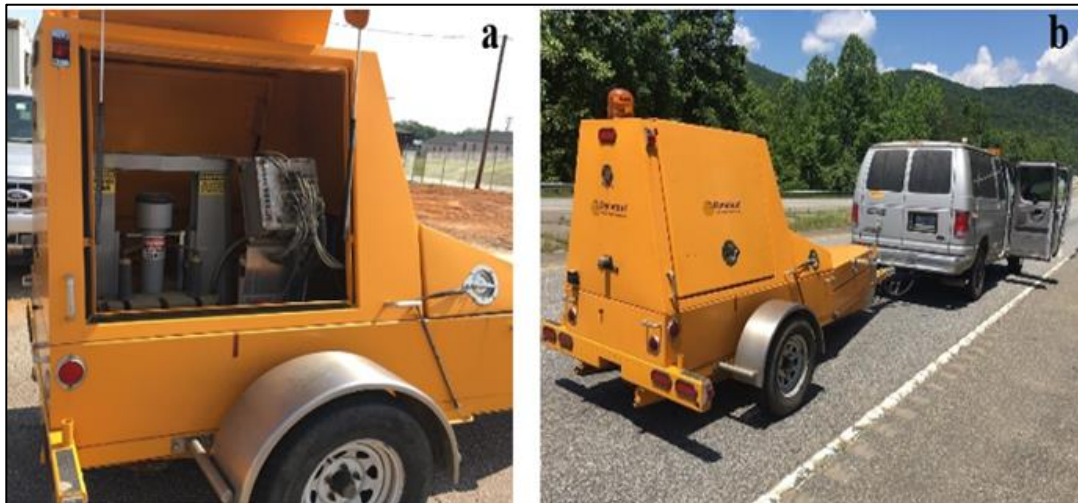
Figure 10 FWD: (a) Loading Frame and (b) System
