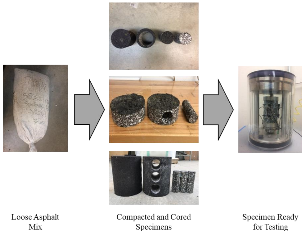
Figure 14 General Process Flow for Preparing Conventional and Small-Scale Dynamic Modulus Test Specimens from Lab and Field Compacted Samples
