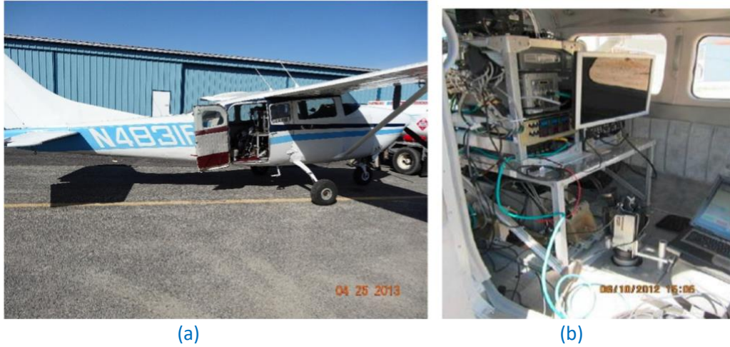
Figure 2. (a) Cessna TP206 research aircraft; (b) Onboard integrated remote sensing system (Source: He et al., 2017)
