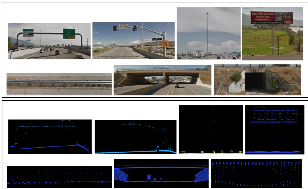
Figure 3. 3D view of large traffic sign, traffic signal, light pole, billboard, barrier, bridge, and culvert in airborne LiDAR (Source: He et al., 2017)
